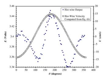
Fig. 4. Hot-wire output and velocity computed from Eq. (6).
