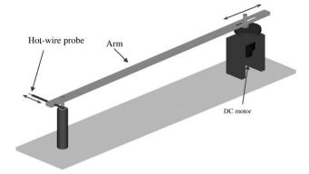
Fig. 1. 3D view of the calibration device.
